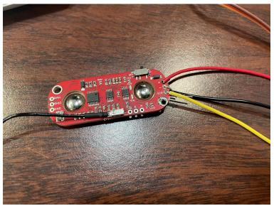
g. Once again, plug the black into the negative side of the breadboard, and the yellow wire into the Arduino/Power Base Shield pin labeled "A0" (Analog 0)
