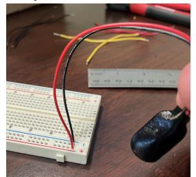
c. Take one of the stripped black wires, connect it to the negative side of the breadboard, and connect the other end to a negative port on the Arduino/Power
